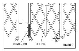
8) With pins raised, extend both halves of gates together to center of opening, mark floor for center pin and drill 3/4" diameter x 3" deep hole Lower pin. Repeat for side pins.
