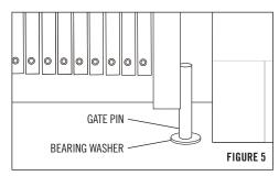
**6)** Extend gate and hang L-bracket on top of gate to verify where it will be mounted. To release tension, lift the wheel 1/2 - 3/4" off the floor. Mark and drill pilot holes into door frame or wall. It may be easier to drill pilot holes if you remove the gate from its floor mount. Place bearing washer and bottom gate pin back into floor mount. Slip "L' bracket over top of gate and 5/16 x 2" lag bolt (not included.) (See Figure 6)
